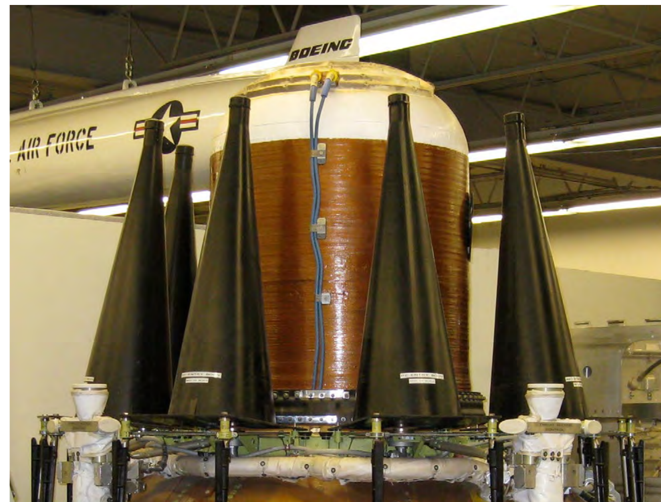
Models of the cone-shaped warheads on a Trident missile at the National Museum of Nuclear Science & History in New Mexico, United States. Published under CC BY-SA 2.0 license.
