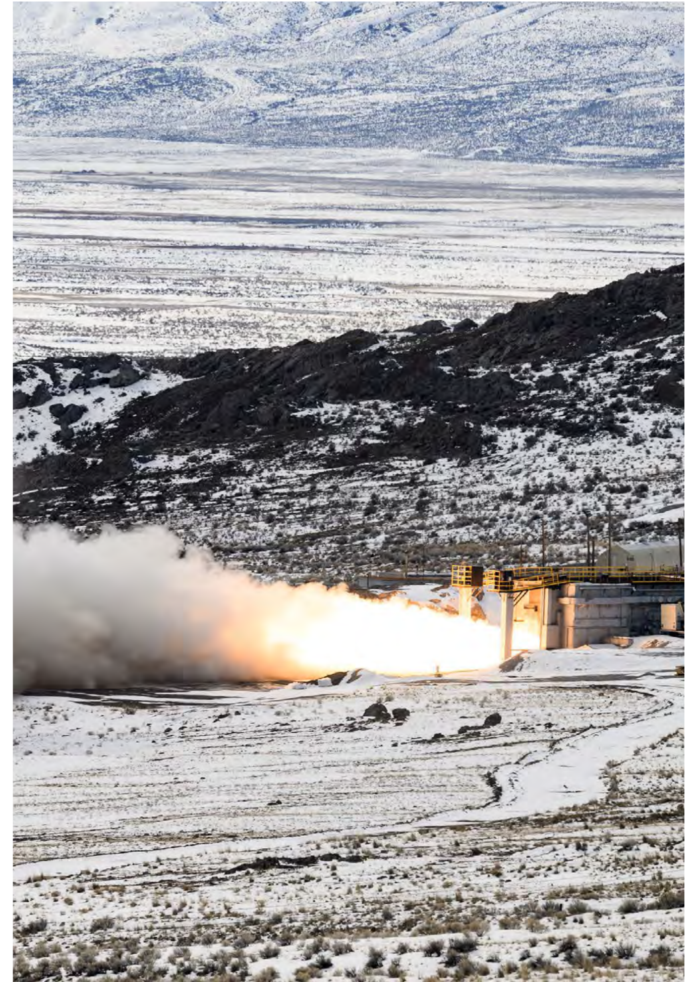
Static fire test for Sentinel solid rocket motor. ©Public Domain.
