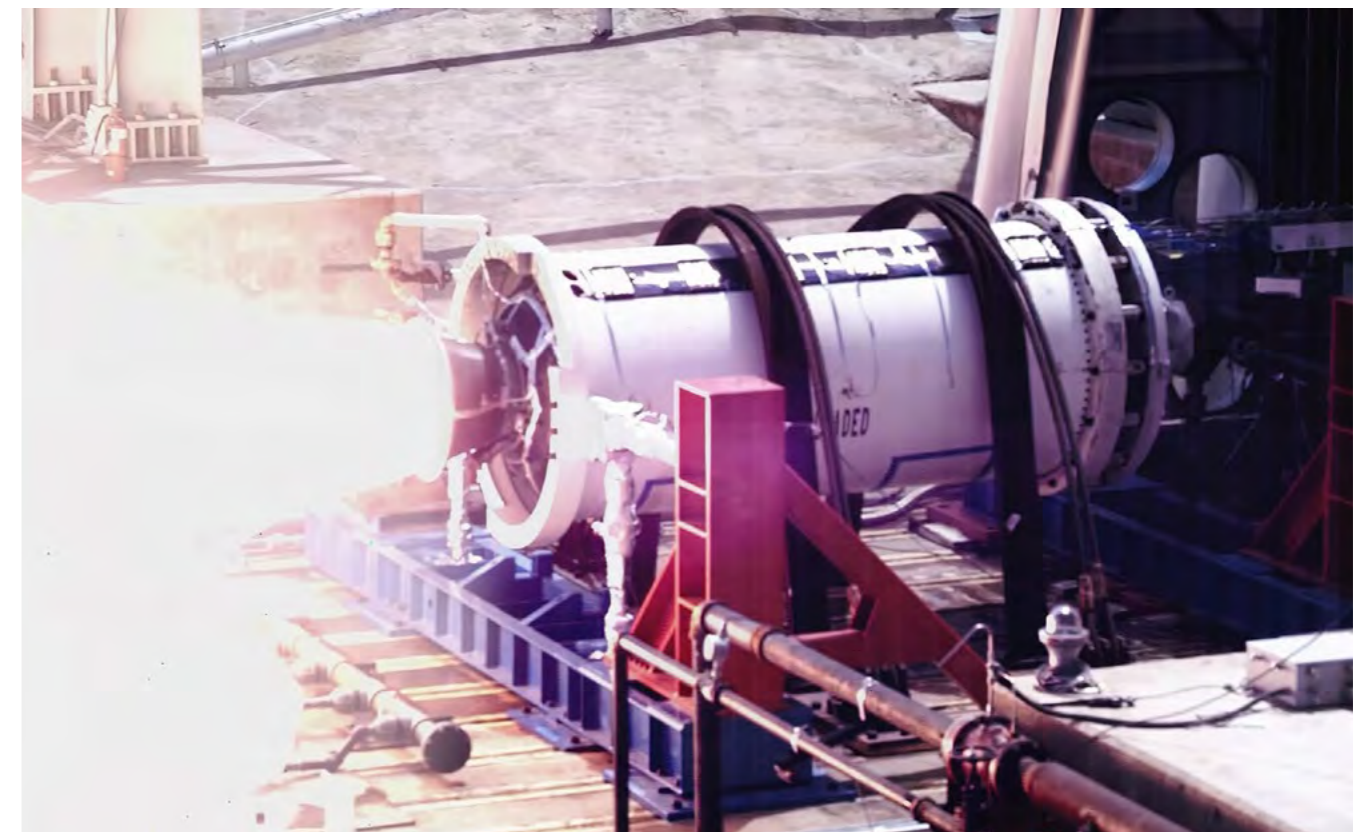
Aerojet Rocketdyne's Design Verification Test of the eSR-19. Source: Aerojet Rocketdyne, Inc.
