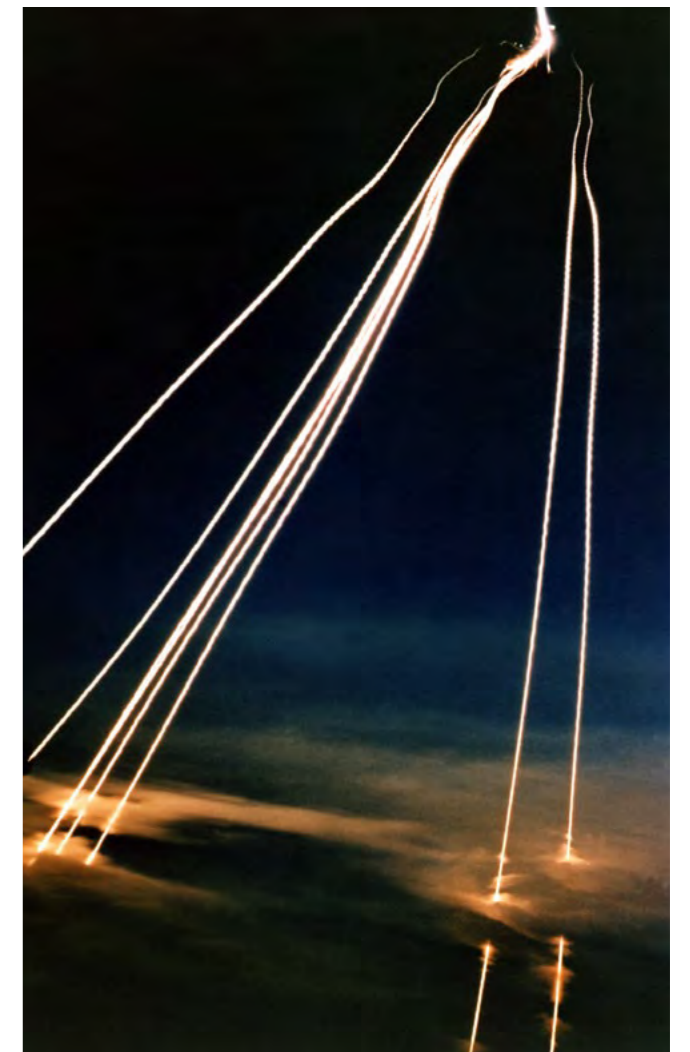
A time exposure of eight Peacekeeper (LGM-118A) intercontinental ballistic missile reentry vehicles passing through clouds while approaching an open-ocean impact zone during a flight test. ©Public Domain.
