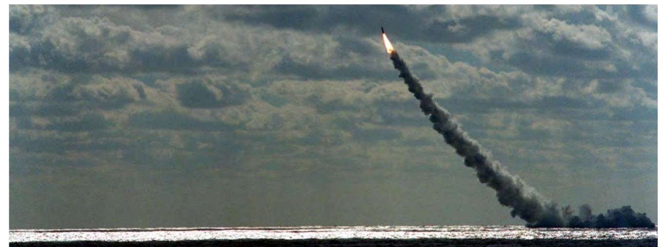
A Trident II D-5 intercontinental ballistic missile lifts off from the water after being launched from the submerged nuclear-powered strategic missile submarine USS TENNESSEE (SSBN-734). ©Public Domain.
